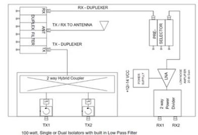
100 watt, Single or Dual Isolators with built in Low Pass Filter
