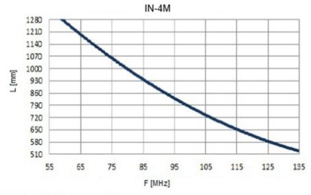
Measured on a Ø 500 mm ground plane
