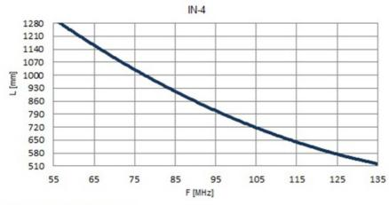
Measured on a Ø 500 mm ground plane
