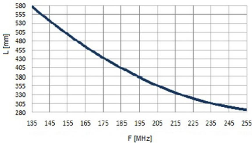
Measured on a  $\varnothing$  500 mm ground plane
