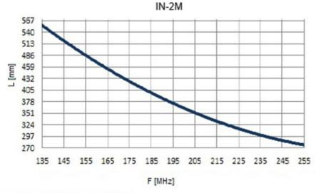
Measured on a Ø 500 mm ground plane
