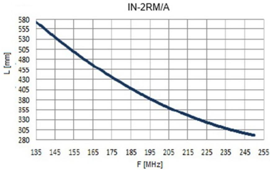
Measured on a  $\varnothing$  500 mm ground plane
