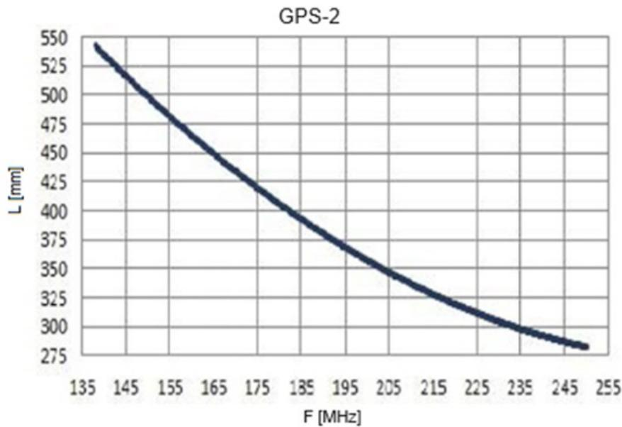
Measured on a  $\varnothing$  500 mm ground plane
