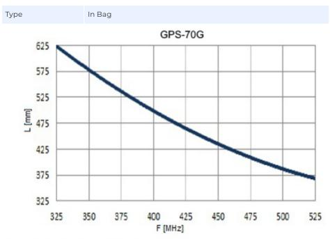
Measured on a Ø 500 mm ground plane
